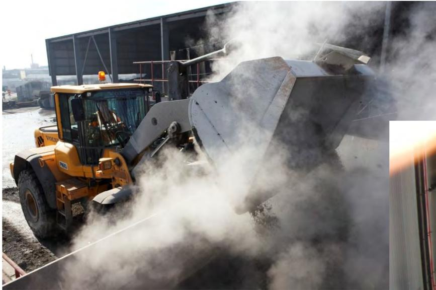
After a few weeks of being stored in the open the IBA is put into a hopper
